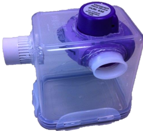
Figure 2.2. Airtight container with Diskus™ inhaler placed inside and INCA™ device attached on top used to measure the acoustic profile, the flow rate and the volume of an inhalation.
